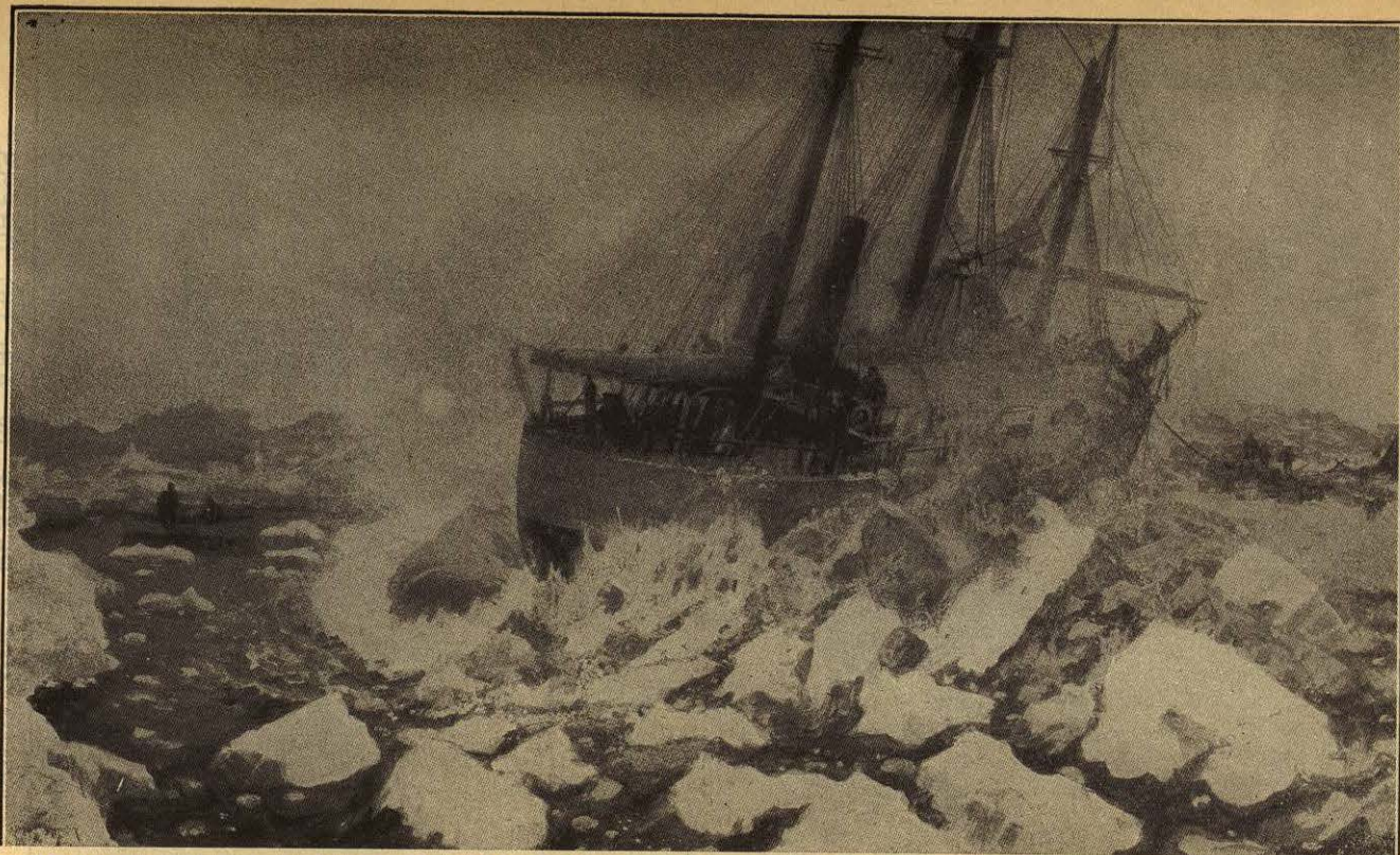
RELEASING A SHIP FROM THE PRESSURE OF AN ICE FLOE—MINE LAID UNDER THE ICE, AND EXPLODED BY ELECTRICITY
