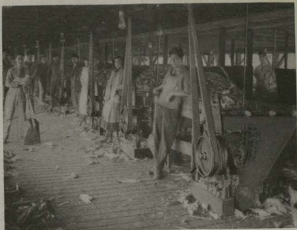
Corn-husking machine; eliminates the drudgery of husking by hand.
