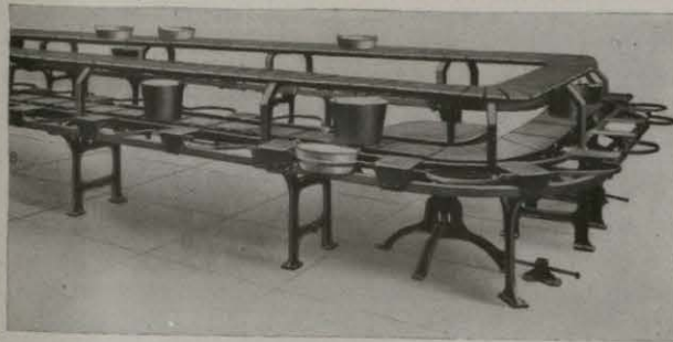
Type of sanitary table on which the buckets or pans are carried to the peelers, and when the preparation is completed, the product and waste are carried away. The pans may be washed after each operation.
