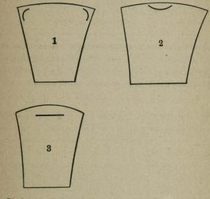
If the axe be cracked as shown in Fig. 1, the corners have been hotter than the middle of the blade; probably by snipping the corners and the middle and comparing the fractures the coarser grain at the corners will tell the tale.
