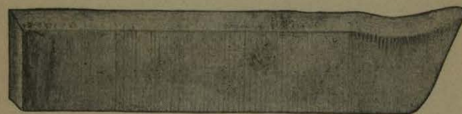
Figure 162. A good tool for heavy cuts.
