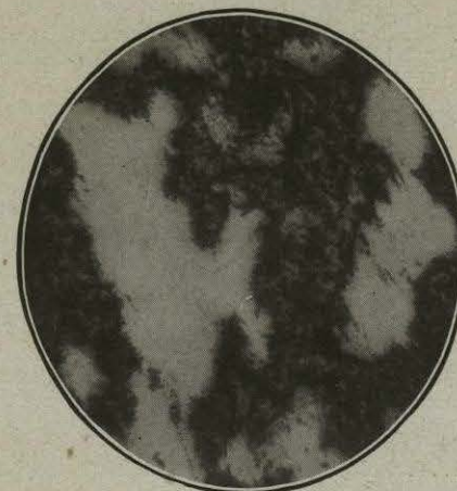
FIG. 119. — Martensite, black. Troostite, white. Magnified 350 diameters.
