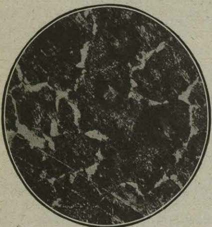
FIG. 117. — Ferrite and sorbite. Magnified 250 diameters.
