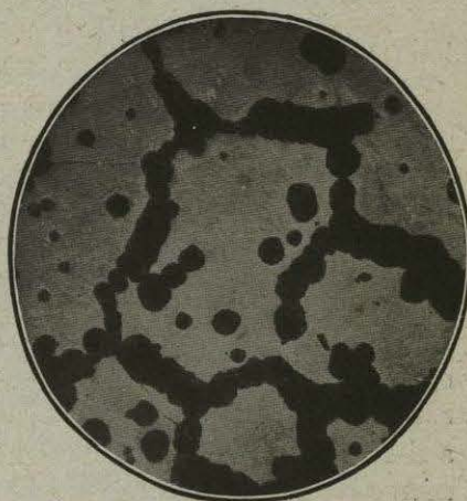
FIG. 118. — Austenite, white. Troostite, black. Magnified 50 diameters.
