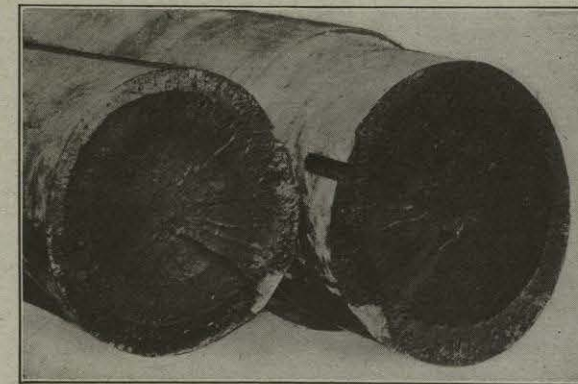
FIG. 60. — Piece forged with relatively light hammer.
