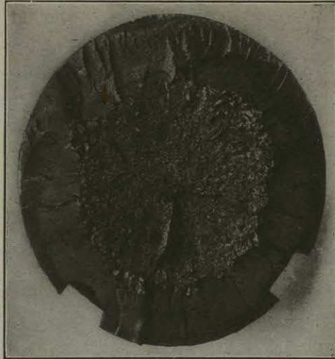
FIG. 58. — Effect of hammer forging.
