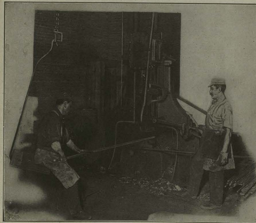
FIG. 30. — Hammering octagon bars.
