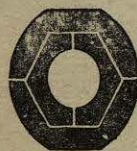
Fig. 559.—Section of Bars used to make Tubes by the Perrins Process.
