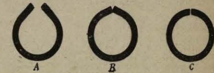
Fig. 556. —Successive Stages in the Formation of a Butt-welded Tube.
