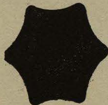
Fig. 524.—Section of Large Ingot for Heavy Forgings.
