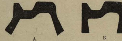
Fig. 385. —Box Tram Rail.—A, in last shaping pass; B, when closed in the finishing pass.
