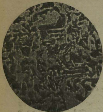
No. 65.—Steel rail as rolled. Interior of heads. Transverse section. Magnification 150 diameters.
