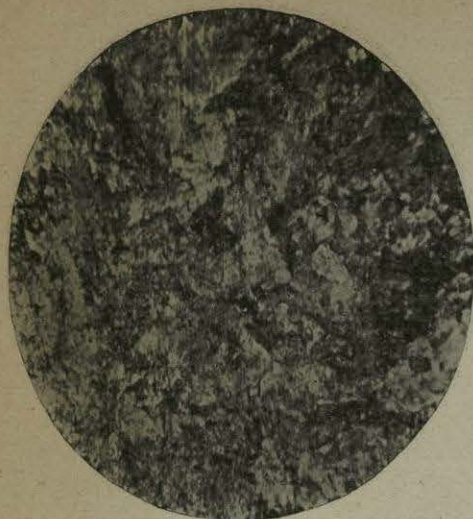
No. 21.—Annealed for 30 minutes at 900° C.; slowly cooled. Pearlite structure not resolved under this power.
