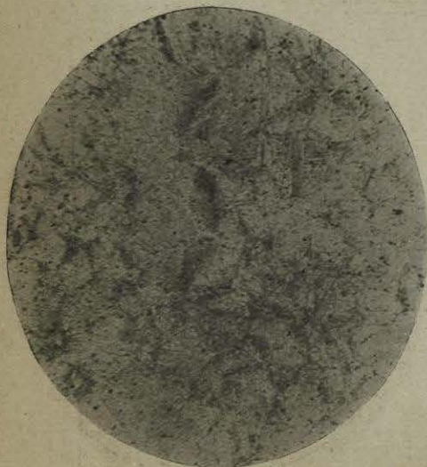
No. 4.—Heated to 900° C. for 30 minutes; quenched in oil from 900° C. Confused structure not resolved under this power.
