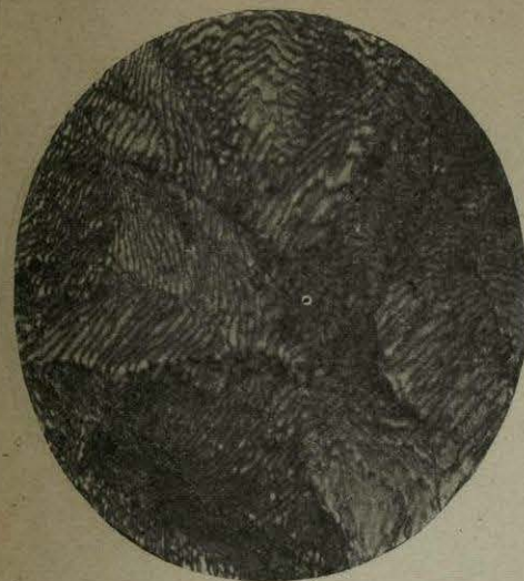
No. 26.—Same section as No. 21. Annealed and slowly cooled. Well-developed Pearlite; saturated steel.
