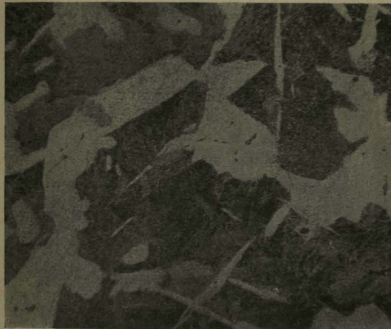
No. 44.—Steel Casting, as cast. Magnification 100 diameters.
