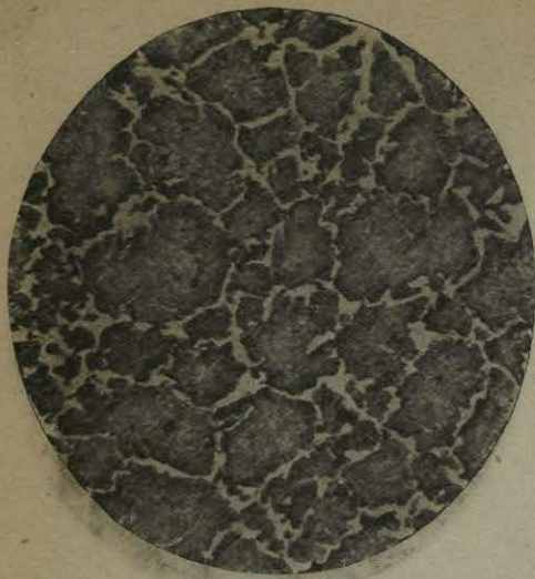
No. 11.—Annealed for 30 minutes at 900° C.; slowly cooled. Pearlite and Ferrite.
