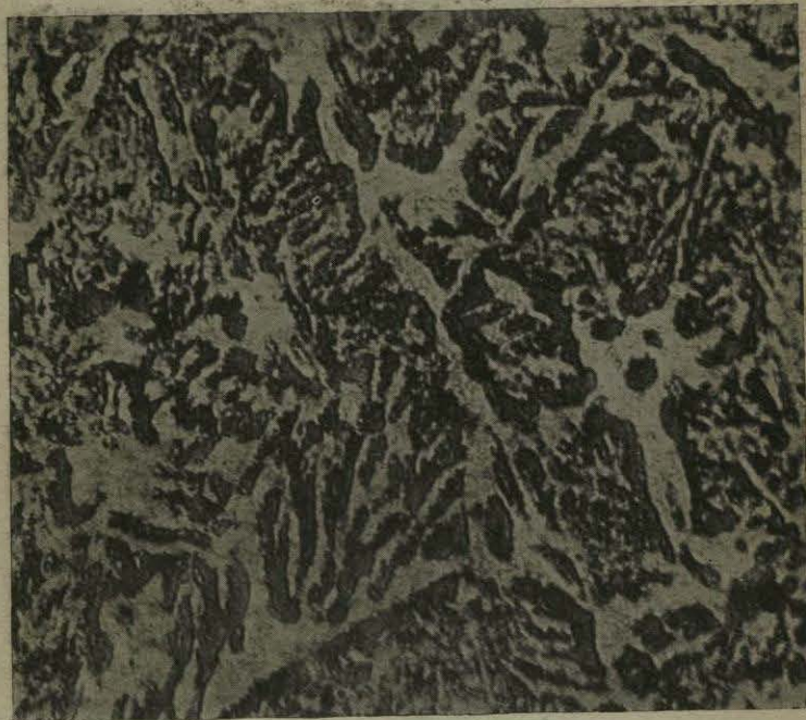
No. 46.—As Cast. Magnification 100 diameters.
