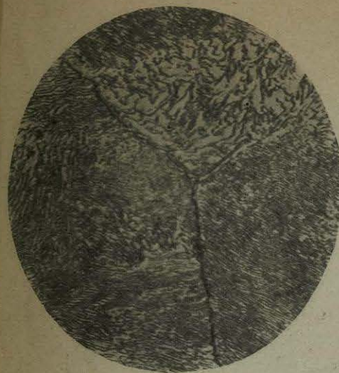
No. 36.—Same section as No. 31. Annealed to 900° C. Well-developed Pearlite and Cementite.
