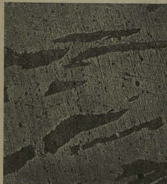
No. 57.—Same bar magnified 150 diameters, after removal from box of Siemens furnace slag, into which it had been dropped when the slag was molten and allowed to remain until the slag was cold.
