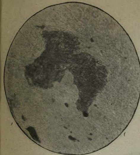
No. 6.—Same section as No. 1, at higher magnification. Annealed for 30 minutes at 900° C.; slowly cooled. Pearlite and Ferrite.
