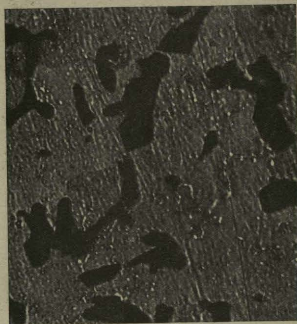
No. 55.—Same bar after heating for 36 hours packed in lime at a temperature of about 1,000° C., and cooling slowly for 32 hours. Magnification 150 diameters.
