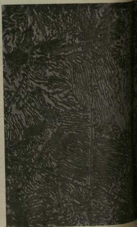
No. 43.—1.5 Carbon Steel from ingot, annealed, showing more segregated Cementite. Magnification 1,000 diameters.
