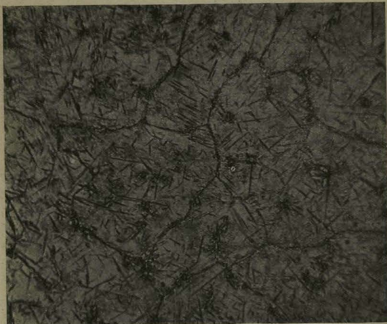
No. 41.—1.5 Carbon from ingot as cast. Magnification 100 diameters.
