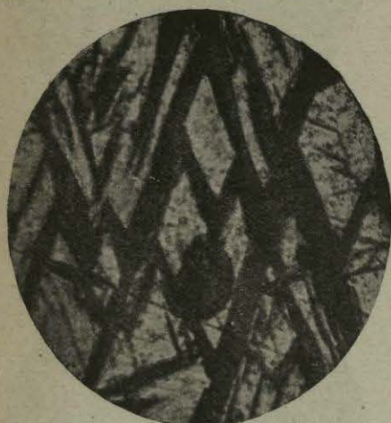
Fig. 283.—Sample of Steel containing 1.6 per cent. of Carbon quenched in Ice Brine from 1,100° C. The light ground mass is Austenite, and the dark barb-like structure Martensite or Hardenite.
