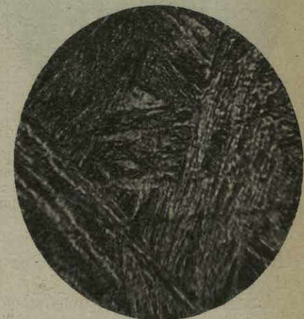
Fig. 282.—Steel containing .468 C quenched from a temperature of 820° C. in water at 15° C. consisting entirely of Martensite. The interlacing crystalline structure is characteristic of Martensite.
