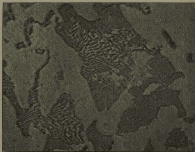
Fig. 256.—Larger percentage of iron than eutectoid mixture. Carbonless iron (Ferrite) in matrix of eutectoid Pearlite.
