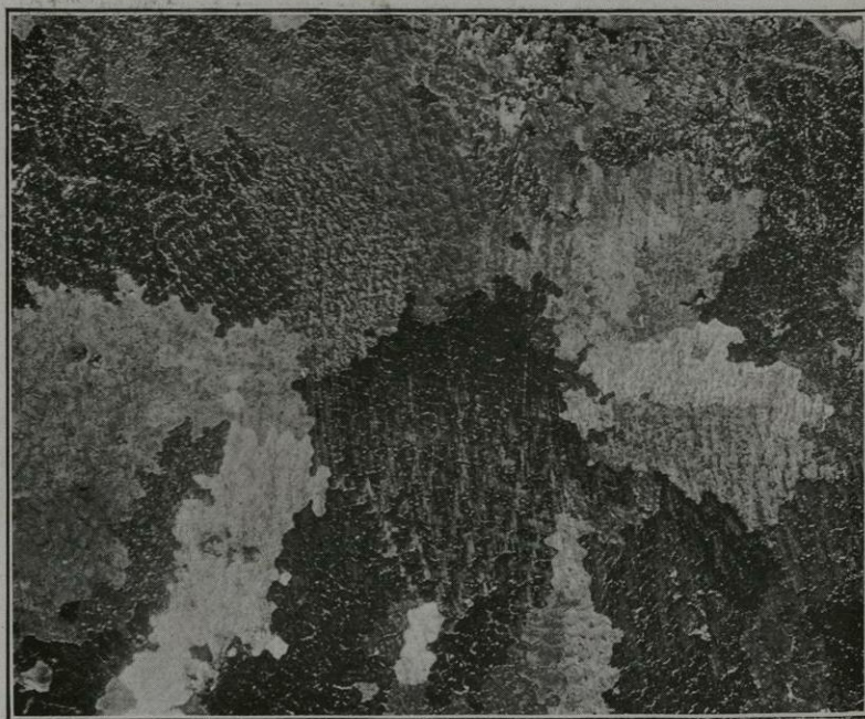
Aluminium-bronze containing 7.5 per cent. of Aluminium. Same as No. 30, but raised to a temperature near its melting-point. \times 10 . No. 31.
