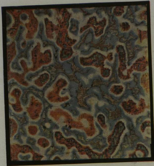
B —Slowly cooled phosphor bronze, heat tinted, showing copper (red), non-homogeneous solution of tin in copper (shading from white to blue-grey) and phosphide of copper (yellow).
