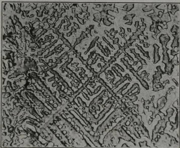
Cast Phosphor-bronze containing 10 per cent. of Tin and 0.7 per cent. of Phosphorus. \times 100 . No. 14.
