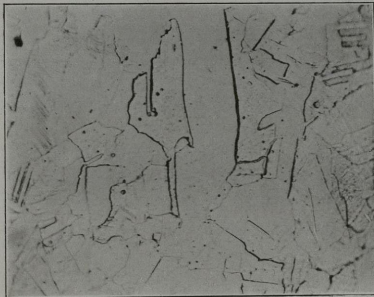
Manganese-bronze Firebox Stay containing 4 per cent. of Manganese. \times 1000 . No. 20.
