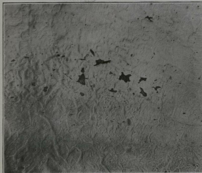
Steel containing Slag polished in Relief. \times 100 . No. 41.
