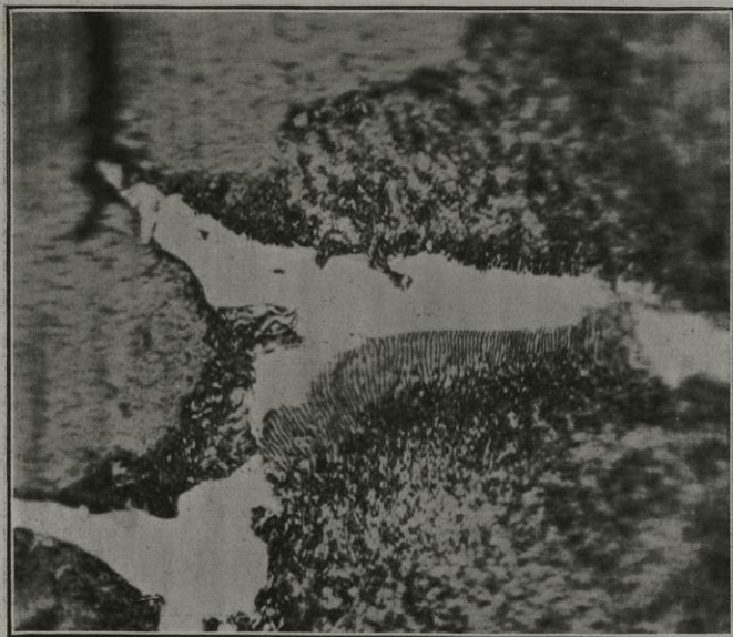
Fringe of Phospho-carbide Eutectic in Grey Iron. \times 1000 . No. 7.
