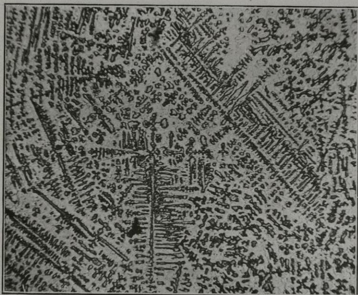
Cast Phosphor-bronze containing 10 per cent. of Tin and 1.5 per cent. of Phosphorus. \times 100 . No. 15.
