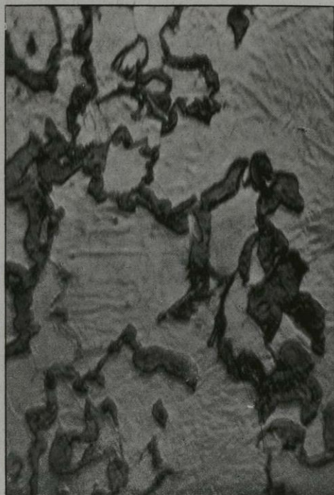
Steel containing 0.45 per cent. of Carbon quenched from 730°. The dark constituent is Troostite.
