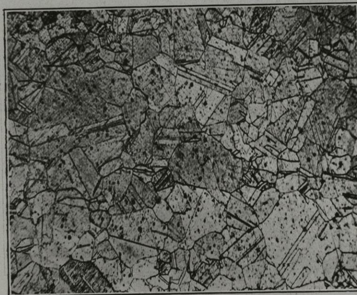
Rolled Brass containing 30 per cent. of Zinc. \times 100 . No. 12.
