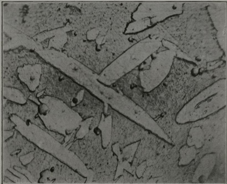
Manganese-bronze, rolled. \times 1000 . No. 22.
