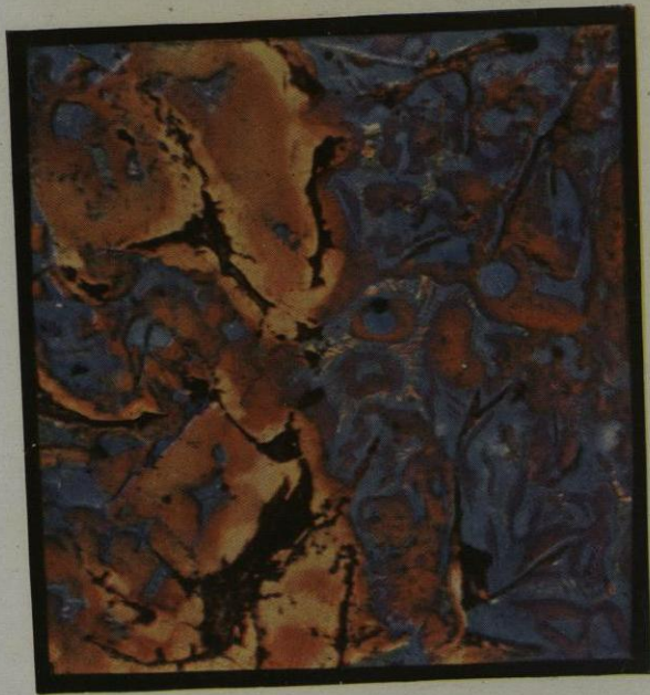
A —Grey Iron containing 2 per cent silicon and 1 per cent phosphorus, heat tinted, showing graphite (black), solid solution of silicon in iron (yellow), and phosphide of iron (blue).
