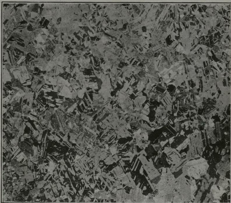
Aluminium-bronze containing 7.5 per cent. of Aluminium. Same as No. 29 after further Annealing. \times 10 . No. 30.
