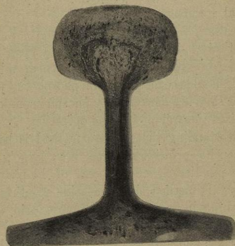
Fig. 189.—Auto-sulphur prints of two rails from different parts of the same ingot. The dark spots represent portions rich in sulphides.
