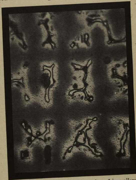
Fig. 172.—Photo-micrograph of a cleavage face of iron alloyed with 2 per cent phosphorus cut from the metal in the cast condition. It was etched with nitric acid, which acted relatively more rapidly on the purer spines, the first to freeze leaving a dark stain. The eutectic of phosphorus and iron containing about 10 per cent. of phosphorus which was the last to freeze is boxed in between the crystallite spines.
