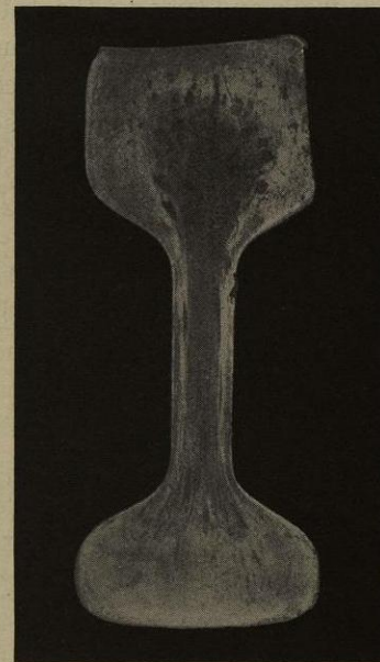
Fig. 184.—Segregated rail broken on the road. The core was unsound and may have been defective before placing on the track. The dark curved line on the right represents a crack.
