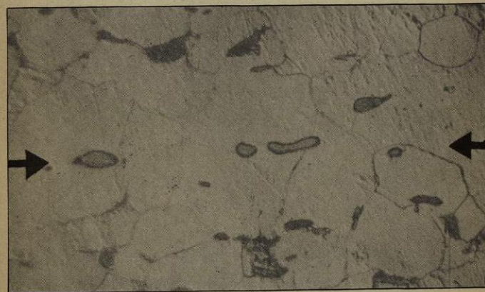
Fig. 187.—Welded-up blowhole cavity containing sulphide inclusions.
