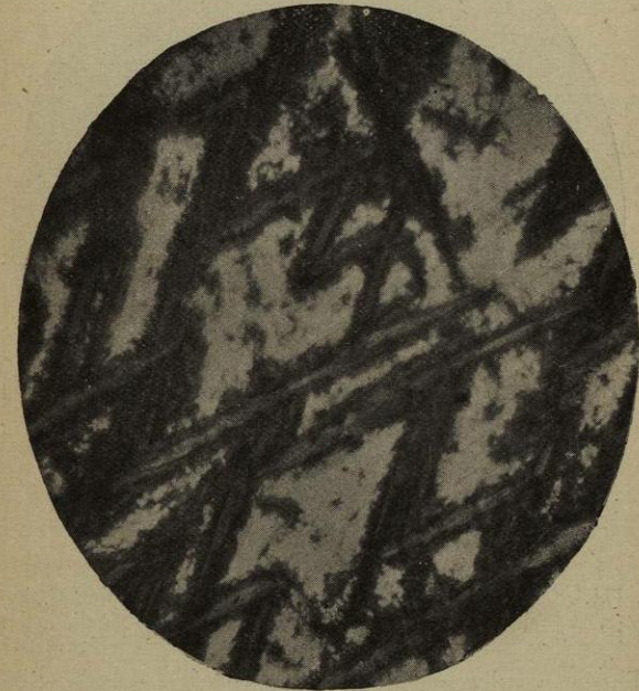
Fig. 170.—CARBON 1·57 per cent. Quenched from 1050° C. in ice water, and reheated to 395° C. Polish-attack. V \times 250 diameters.
