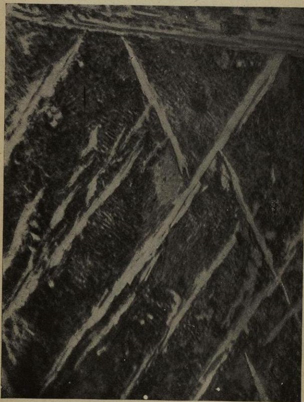
Fig. 169.—CARBON 1.57 per cent. Cemented steel drawn from a cementation furnace and cooled in air. Polish-attack. V \times 1000 diameters.
