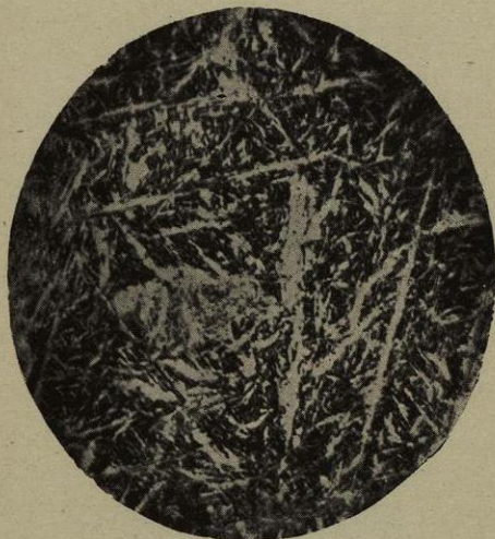
Fig. 168.—CARBON 1.25 per cent. Quenched from 1050^{\circ} C. Polish-attack. V \times 250 diameters.
