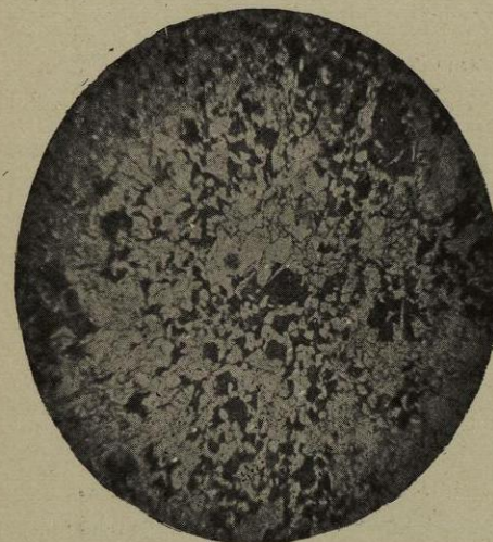
Fig. 162.—CARBON 0.45 per cent. Quenched from 650° C. Etched with 20 per cent. nitric acid. V \times 100 diameters.
