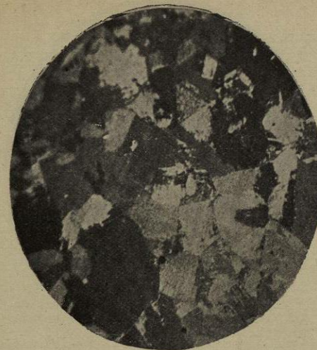
Fig. 156.—CARBON 0.45 per cent. Reheated to, and quenched from, 1225° C. Polish-attack and nitric acid. Oblique illumination. \times 20 diameters.
