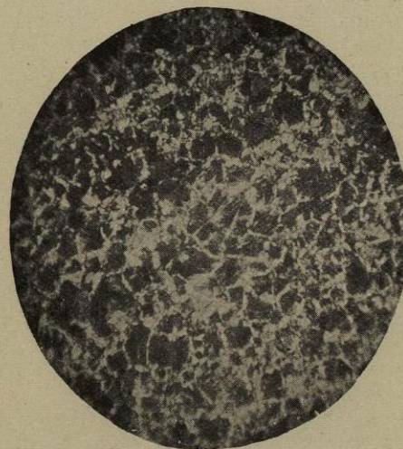
Fig. 145.—CARBON 0.14 per cent. Reheated to 1000° C., and quenched in water at 15° C. Polish-attack. Iodine or nitric acid. V \times 100 diameters.
