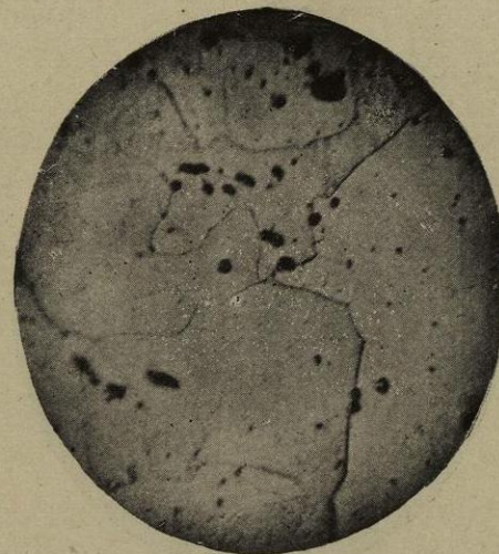
Fig. 136.—IRON (0·02 per cent. carbon). Etched with iodine. V \times 100 diameters.
