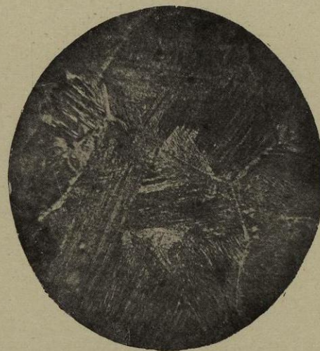
Fig. 147.—CARBON 0.14 per cent. Reheated to 1340^{\circ} C., and quenched in water at 15^{\circ} C. Etched with 20 per cent. nitric acid. Oblique illumination. \times 100 diameters.
