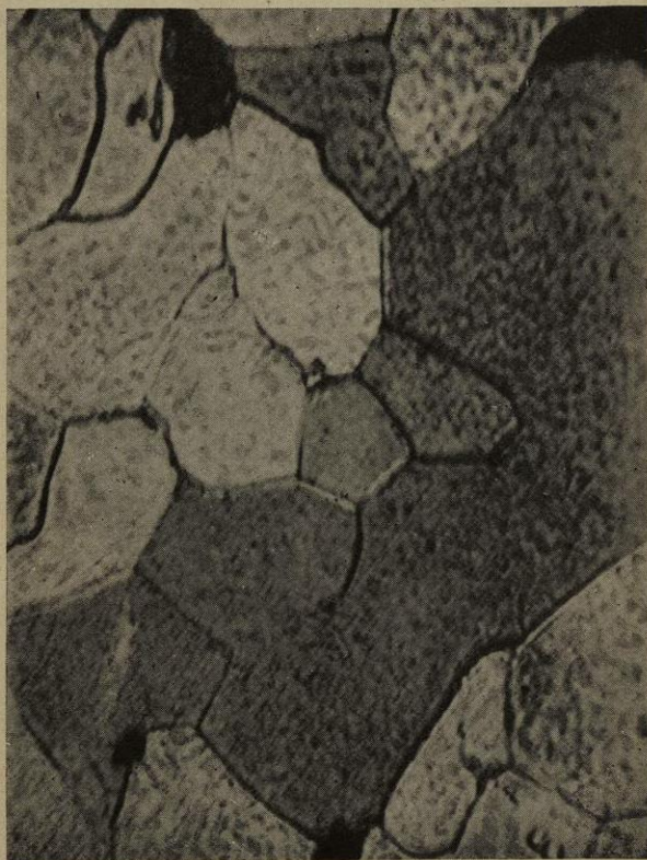
Fig. 139.—CARBON 0.14 per cent. Etched with tincture of iodine. V \times 100 diameters.
