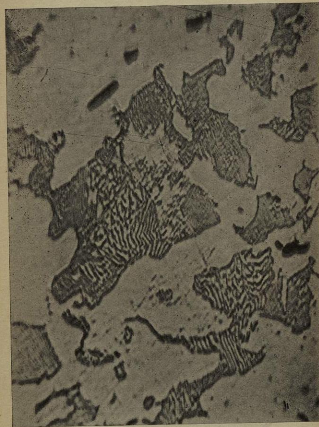
Fig. 148.—FORGED STEEL. CARBON 0·45 per cent. Polish-attack. V \times 1000 diameters.
