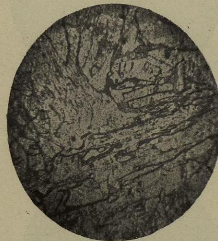
Fig. 142.—CARBON 0.14 per cent. Reheated to 1330^{\circ} C. Etched with 20 per cent. nitric acid. V \times 100 diameters.
