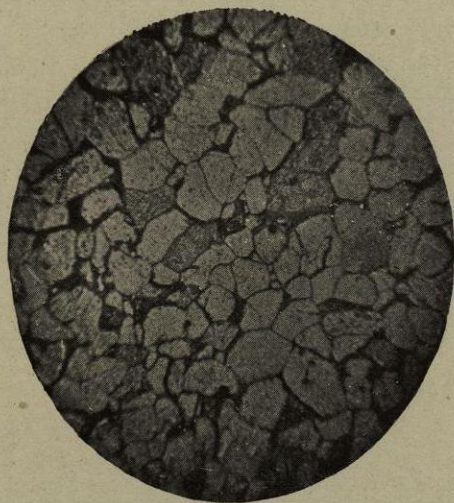
Fig. 141.—CARBON 0.14 per cent. Reheated to 1015^{\circ} C. Etched with 20 per cent. nitric acid. V \times 100 diameters.
