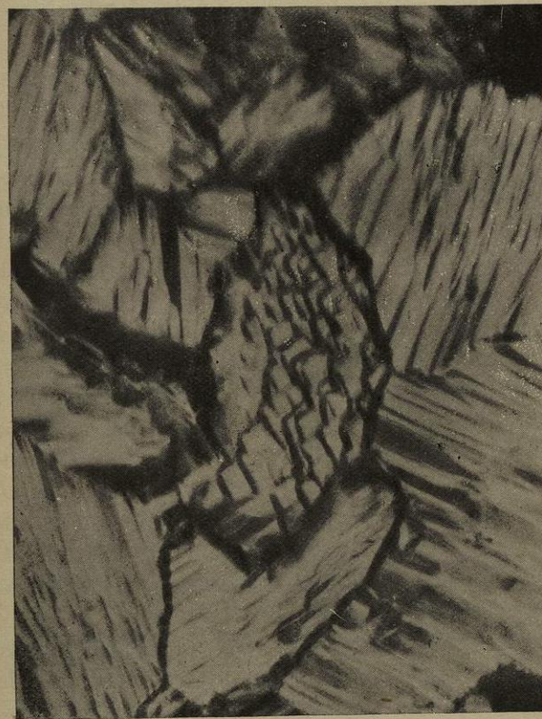
Fig. 124.—FERRITE. Strongly etched. Showing the orientation of the crystals. V \times 400 diameters.
