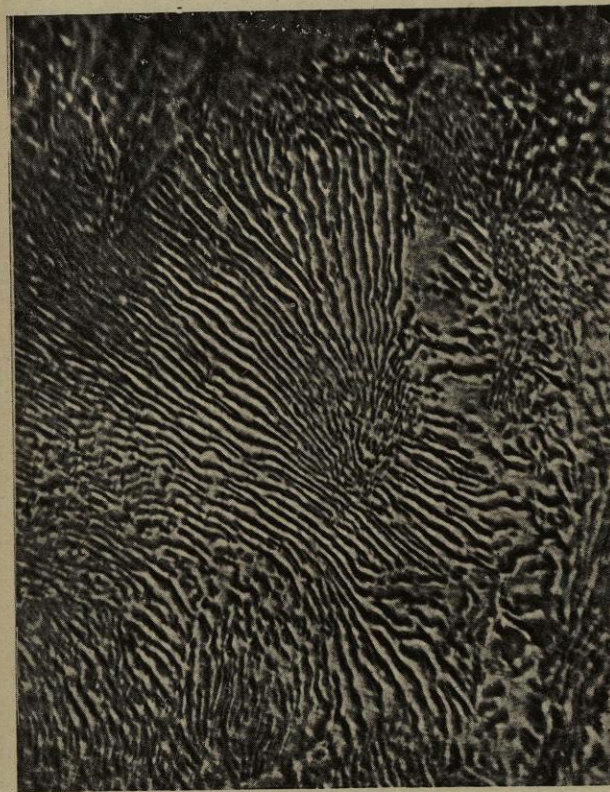
Fig. 127.—PEARLITE in 1.00 per cent. carbon steel. Forged, heated, and cooled slowly from 800^{\circ}C . Polished only. V \times 1000 diameters.
