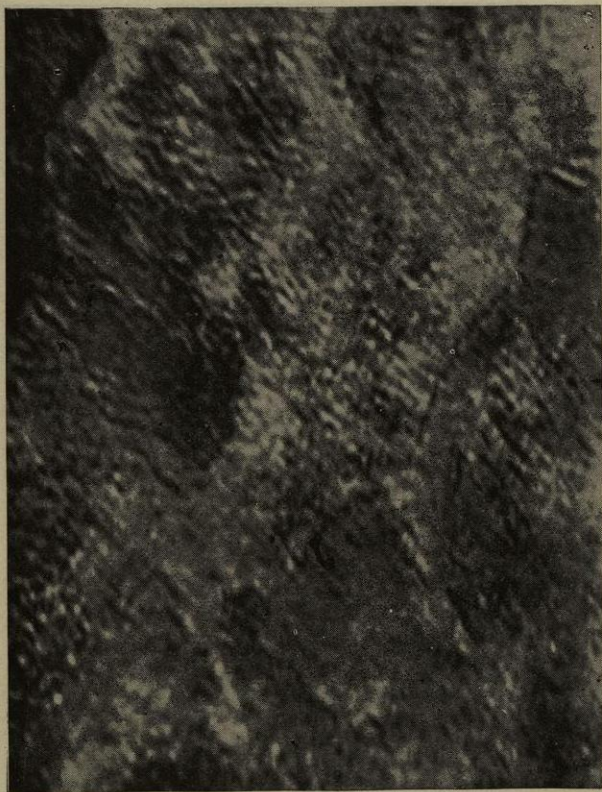
Fig. 129.—SORBITIC PEARLITE (granular) in 1.00 per cent. carbon steel. Polish-attack. V \times 1500 diameters.
