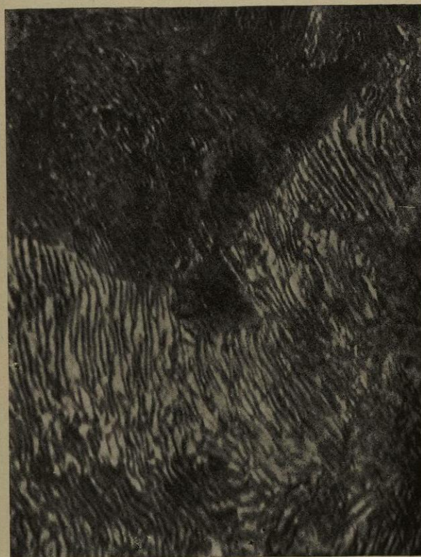
Fig. 130.—PEARLITE passing into SORBITE in 1.00 per cent. carbon steel. Polish-attack. V \times 1500 diameters.
