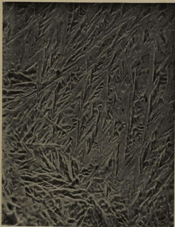
Fig. 135.—AUSTENITE STEEL after plain polishing and placing in liquid air revealing the transition to MARTENSITE. V \times 250 diameters. ( Typical martensite structure. )
