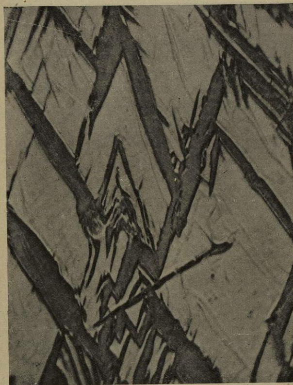
Fig. 134.—AUSTENITE and HARDENITE in 1.57 per cent. carbon steel. Polish-attack. V \times 1000 diameters.
