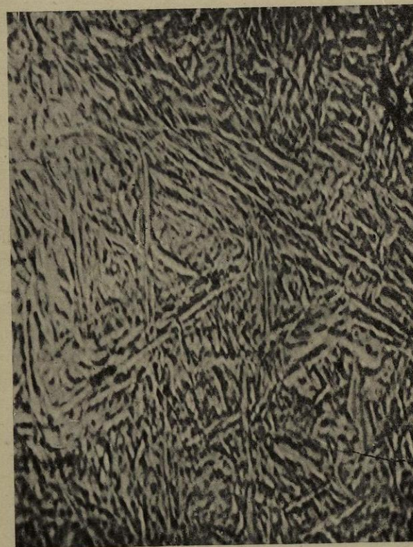
Fig. 131.—MARTENSITE in 0.45 per cent. carbon steel. Polish-attack. V \times 1000 diameters.
