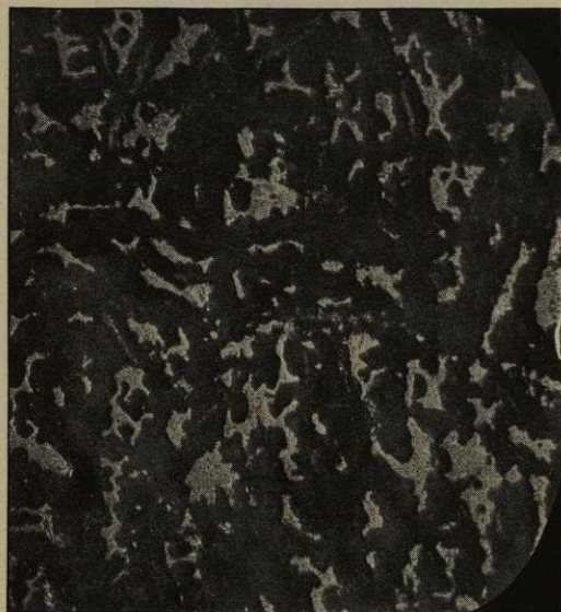
Fig. 116.—Phosphide of iron eutectic in pig-iron containing 1.5 per cent. phosphorus.
