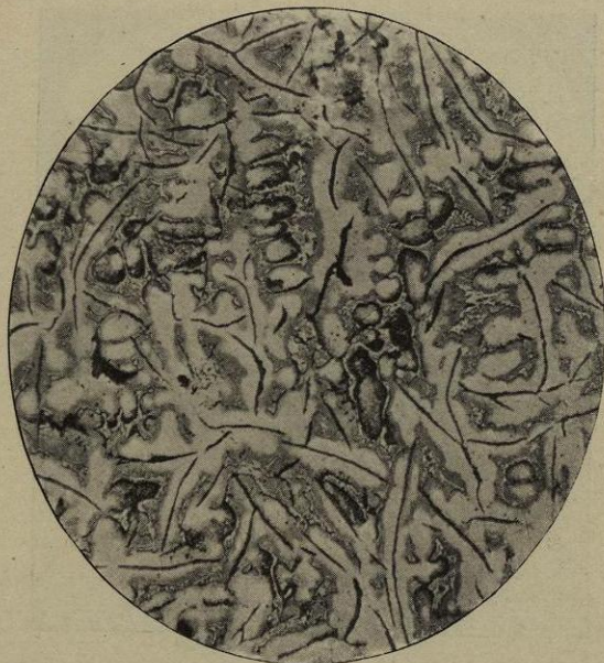
Fig. 120.—Pig-iron containing 0.4 per cent. combined carbon.
