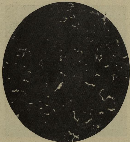
Fig. 118.—Phosphide of iron eutectic in pig-iron containing 0.3 per cent. phosphorus.
