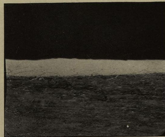
Fig. 107.—Crown wire of a winding rope made brittle by friction heat and rapid cooling. The white band is martensite. \times 50 .
