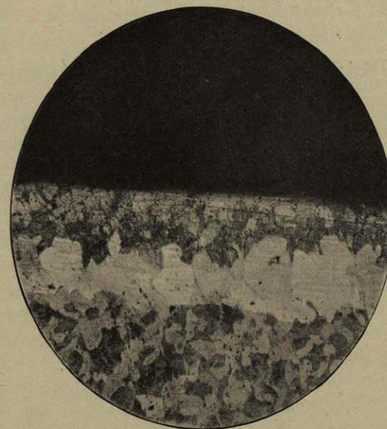
Fig. 123.—Malleable casting, showing evidence of recarburisation on the outside layer which made the casting weak. \times 50 .
