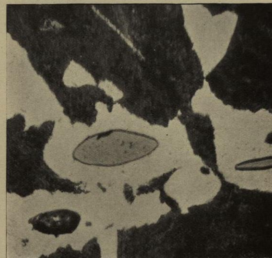
Fig. 111.—Steel casting which had been slightly forged. Note the ovoidal form of the manganese sulphide. \times 300 .
