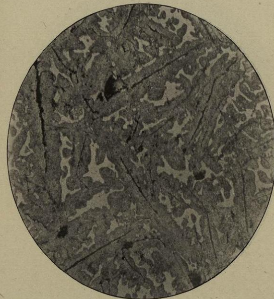
Fig. 121.—Pig-iron containing 0.8 per cent. combined carbon. Ground mass is pearlite. The white patches are iron phosphorus eutectic. Note that the half-tone portions representing pearlite are proportional to the combined carbon. In fig. 119 it is very little, in fig. 120 it is greater, while in fig. 121 all the ground mass is pearlite. Ferrite decreases as the pearlite increases, and the ferrite develops in the direction from graphite to the phosphorus eutectic.
