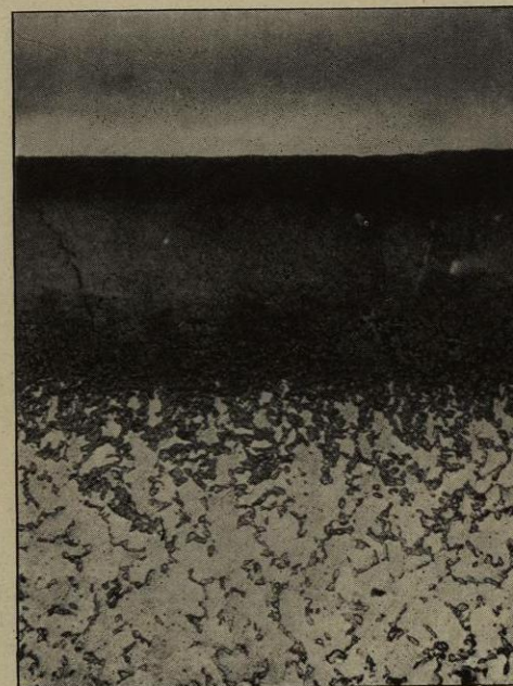
Fig. 113.—Case-hardened motor gear wheel strongly etched with strong acid, showing depth of carburised layer (dark) and that the steel below contains very little carbon. In the best gear wheels the carburised layer is much thicker than that shown in this example. \times 35 .
