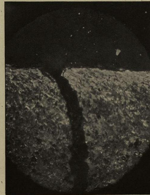
Fig. 101.—Side of a drill hole in a boiler plate which cracked when in use. Note that the line of fracture follows the laminations produced by the drill. \times 250 .
