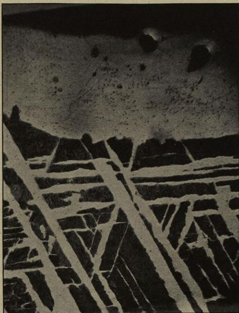
Fig. 104.—Large steel casting with thick decarburised envelope and coarse crystalline structure. It had probably been annealed at a low temperature. \times 50 .
