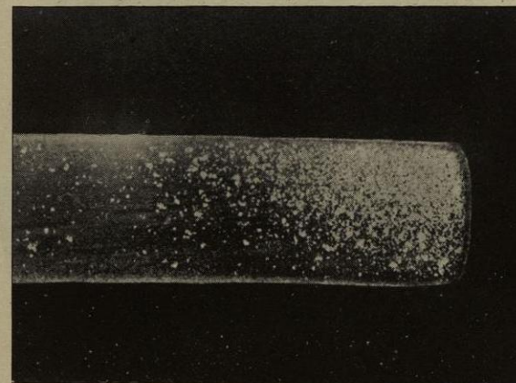
Fig. 105.—Wire rod improperly treated during the patenting process. The white areas are martensite, the dark ground-mass troostite passing into sorbite.
