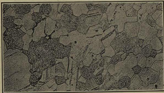
Fig. 85.—Crystallised Iron (Stead), showing differential incrustation revealed by cuprous ammonium chloride etching. \times 150 .
