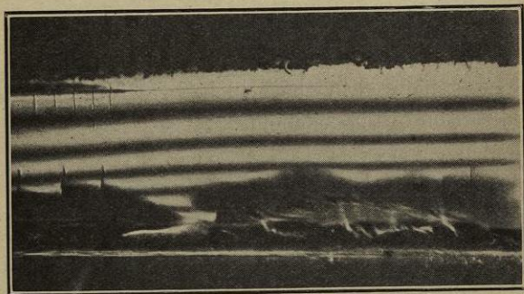
Fig. 53.—Glass cut by diamond scratch and cracked. \times 125 .
