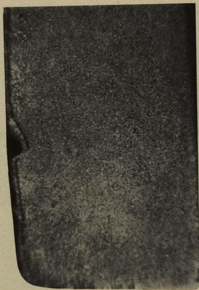
Fig. 41.—GOLD, containing 0.2 per cent. Antimony, reheated to nearly 250°. Etched by nitro-hydrochloric acid. \times 17 diameters.
