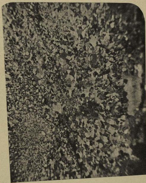
Fig. 39.—GOLD, containing 0.2 per cent. Bismuth, reheated to nearly 250°. Etched by nitro-hydrochloric acid. V \times 17 diameters.
