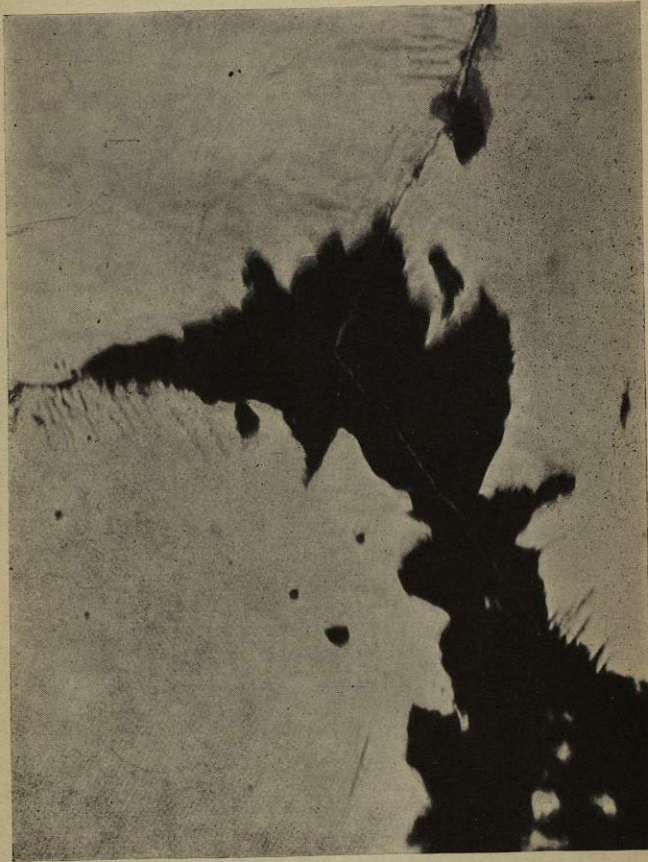
Fig. 37.—CINDER IN A STEEL. Polished. V \times 1000 diameters.
