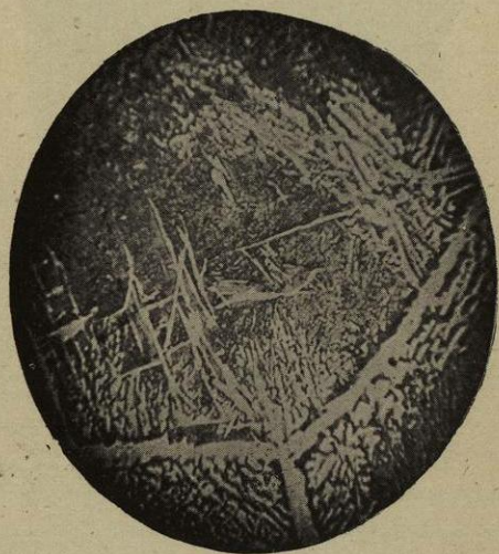
Fig. 44.—FORGED STEEL (0.45 per cent. carbon). Reheated to 1390°. Polish-attack. \times 100 diameters.
