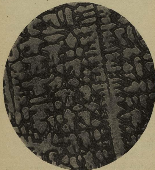
Fig. 32.—BRONZE, with 19 per cent. Tin, cast in sand. Heat, oxidation tinted. V \times 100 diameters.
