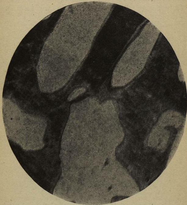
Fig. 35.—BRONZE, with 19 per cent. Tin, quenched from dark red in water at 50^{\circ} . Heat, oxidation tinted. V \times 500 diameters.
