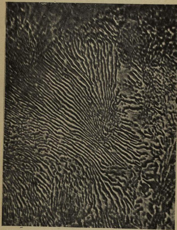
Fig. 20.—FORGED STEEL (1.00 per cent. carbon). Reheated to 800°. Polished in bas-relief. V × 1000 diameters.
