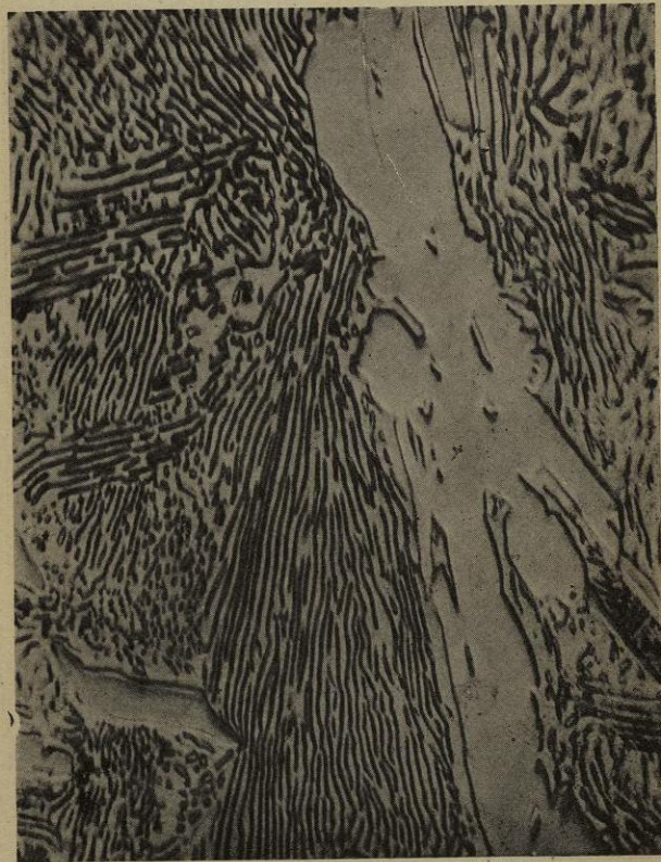
Fig. 21.—CEMENT STEEL (1.57 per cent. carbon). Polish-attack. V × 1000 diameters. (Typical laminated pearlite.)
