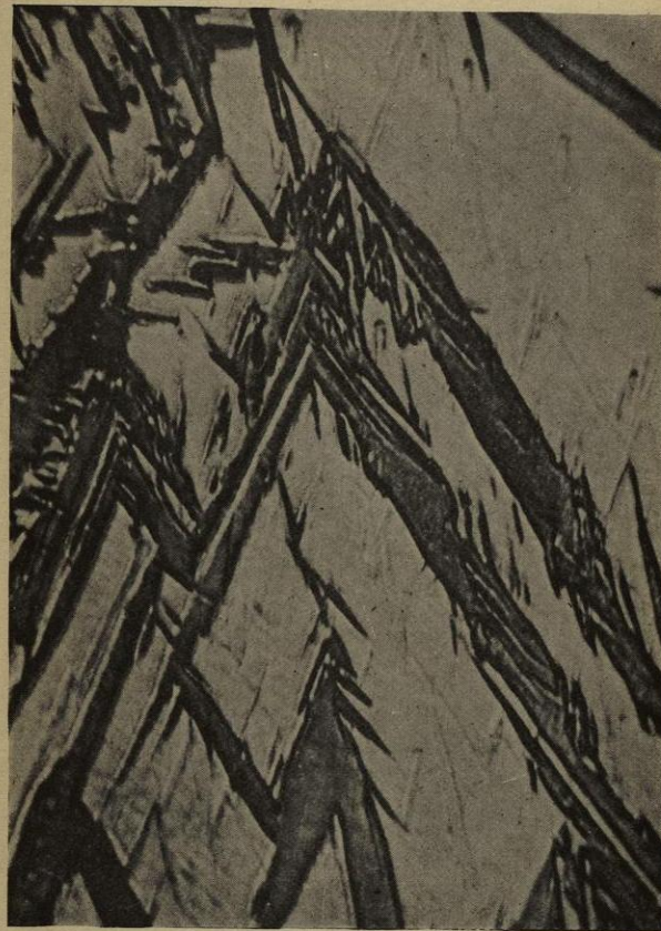
Fig. 23.—CEMENT STEEL (1.57 per cent. carbon). Heated to nearly 1050°, and quenched in ice-cold water. Polish-attack. V \times 1000 diameters.
