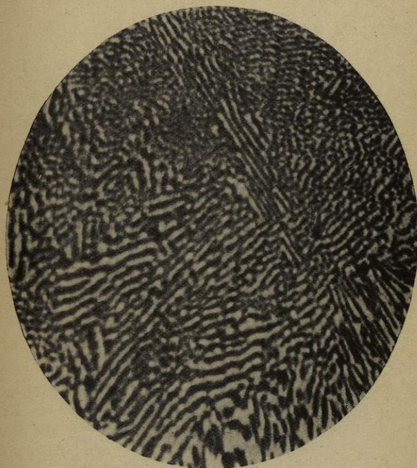
Fig. 14.—COPPER = 28 per cent. ; SILVER = 72 per cent. (Cast.) Heat, oxidation tinted. \times 1000 diameters.
