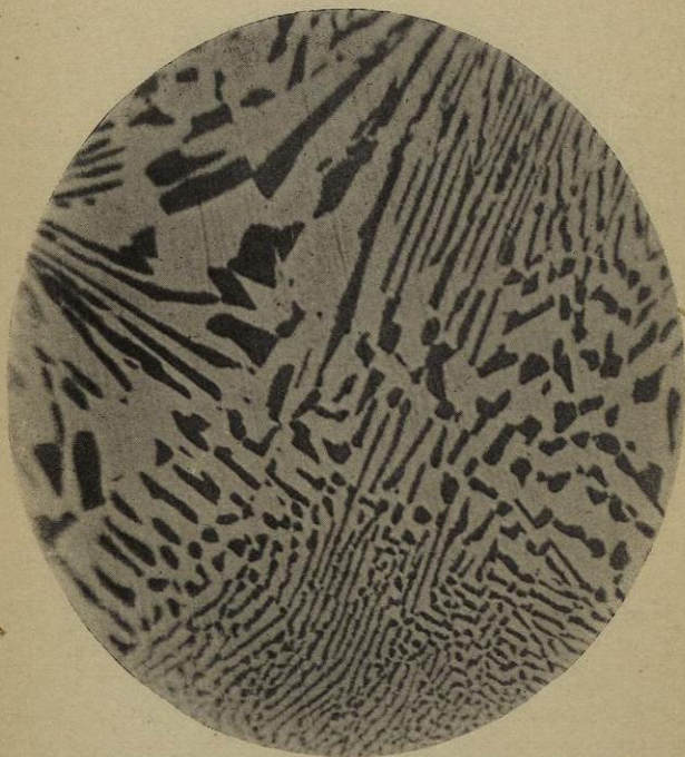
Fig. 15.—COPPER=28 per cent. ; SILVER=72 per cent. (Cast.) Heat, oxidation tinted. \times 600 diameters.
