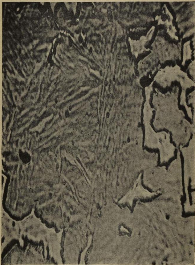
Fig. 24.—FORGED STEEL (0.30 per cent. carbon). Heated to 900°, and quenched at 720°. Polish-attack. V \times 1000 diameters.
