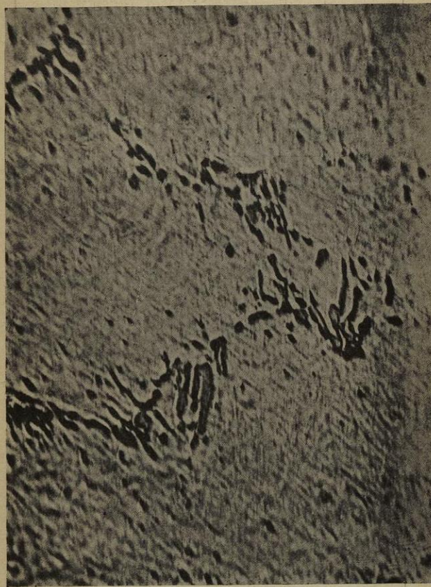
Fig. 25.—FORGED STEEL (1.24 per cent. carbon). Heated and quenched at 735°. Polish-attack. V \times 1000 diameters.
