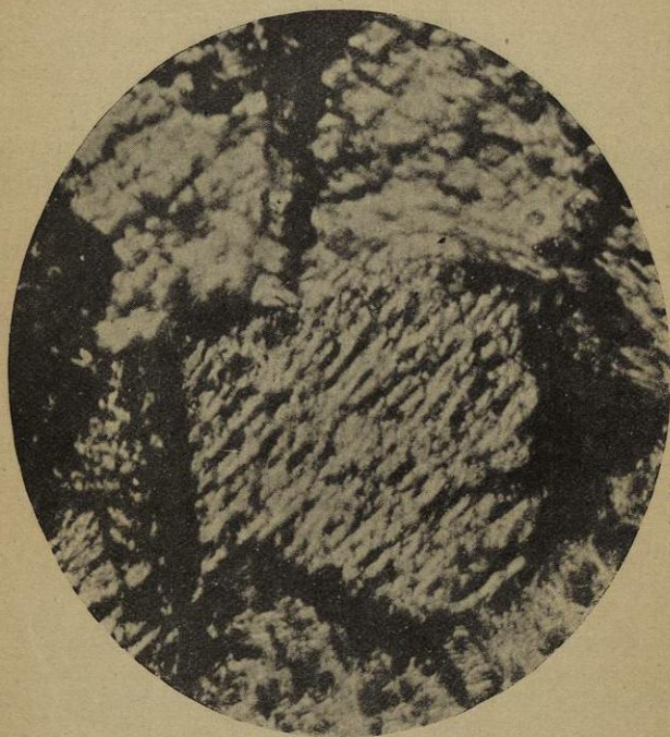
Fig. 5.—HAMMERED MILD STEEL (0.125 per cent. carbon). Attacked by dilute sulphuric acid. \times 1000 diameters.
