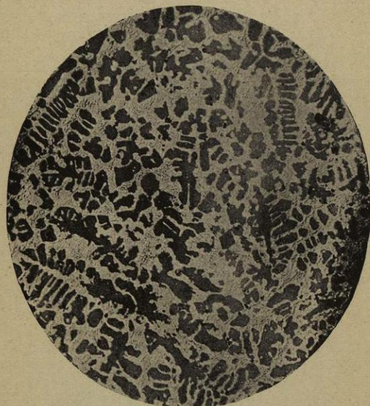
Fig. 6.—GOLD=85 per cent. ; ALUMINIUM=15 per cent. Cast. Polished only. \times 1000 diameters.
