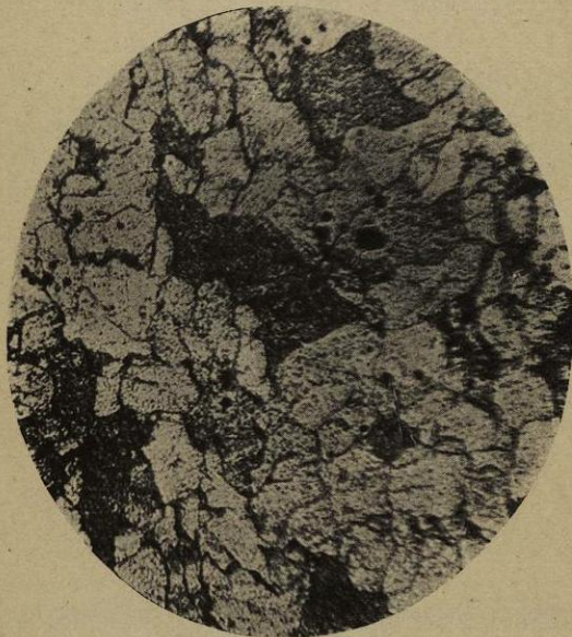
Fig. 3.—HAMMERED MILD STEEL (0.125 per cent. carbon). Attacked by dilute nitric acid. \times 100 diameters.
