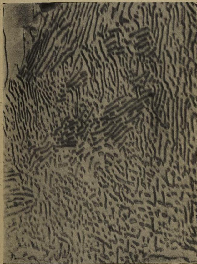
Fig. 1.—CEMENTATION STEEL. Polish-attack. 1 V × 1200 diameters.
