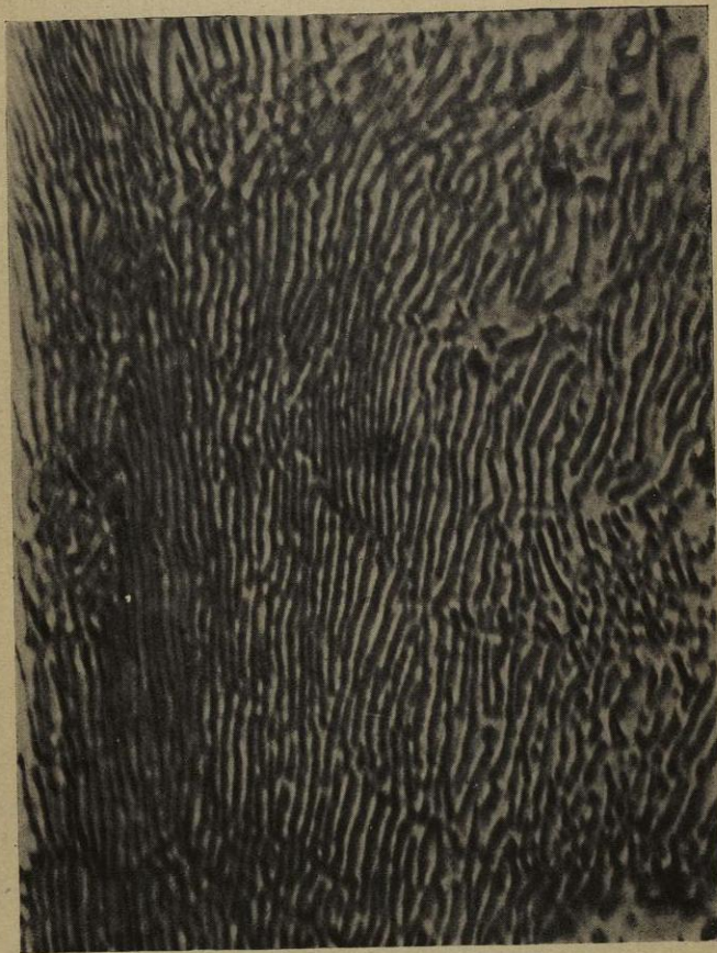
Fig. 11.—CEMENTATION STEEL. Polish-attack. \times 1500 diameters. (Typical lamellar pearlite.)
