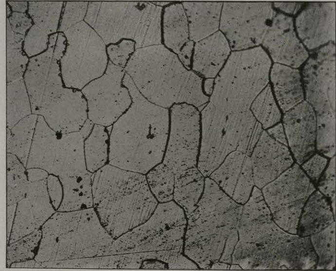
FIG. 102. — Crystals of Ferrite.
