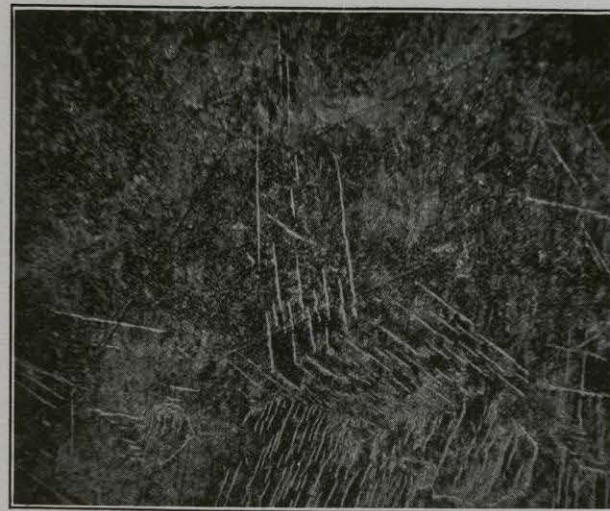
FIG. 99.—Cemented Carbon Steel. \times 100 d.
