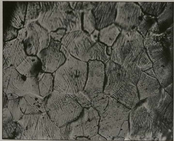
FIG. 103. — Slip-Bands in Ferrite Crystals.
