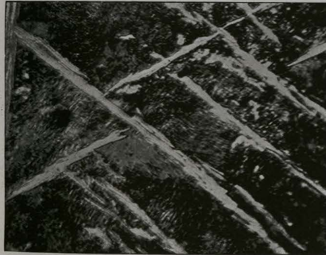
FIG. 54.—1.5 C. Steel, cooled in air, showing Sorbitic Pearlite and Cementite.
