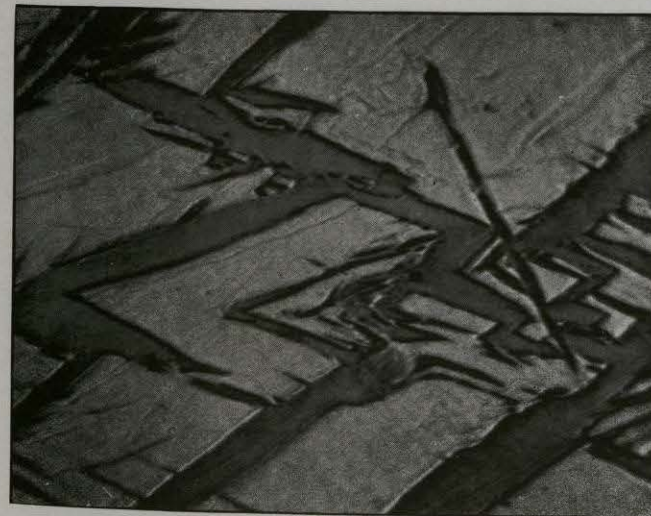
FIG. 55.—1.5 C. Steel. Quenched at 1000° in iced water, showing Austenite and Martensite.
