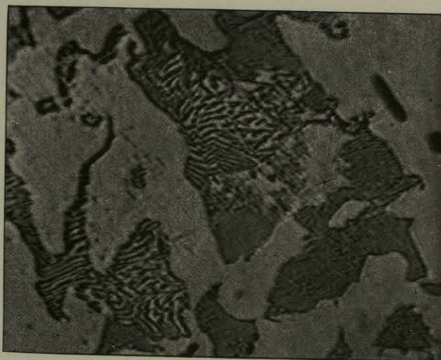
FIG. 48.—0.45 C. Steel. Annealed, showing Pearlite and Ferrite.
