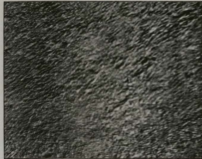
FIG. 51.—Same as above, but tempered after quenching.
