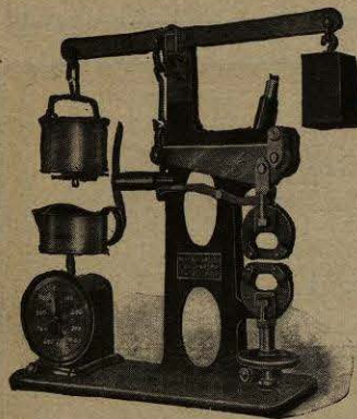
Apparatus according to Jackson for Specific Gravity of Cement.
