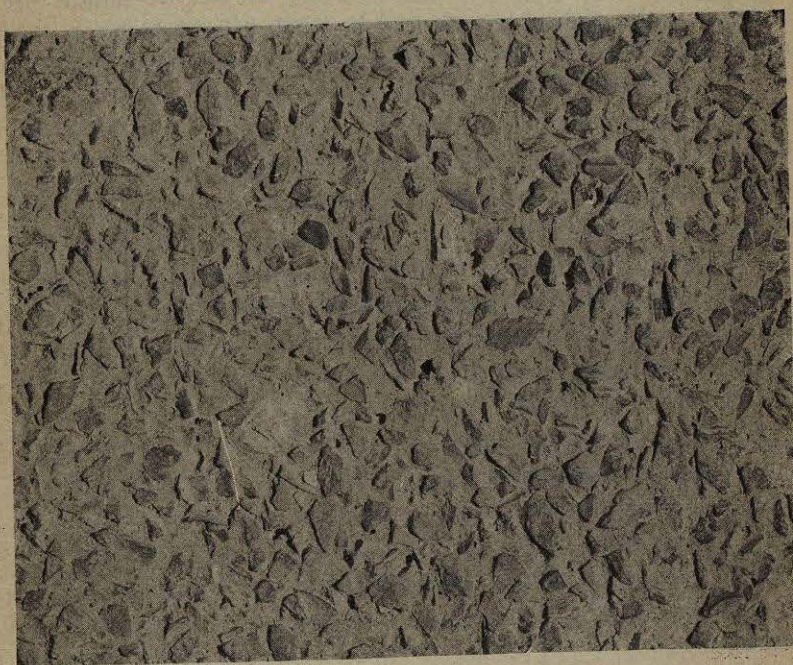
FIG. 106.—Surface of Washed Concrete. (See p. 289.)
