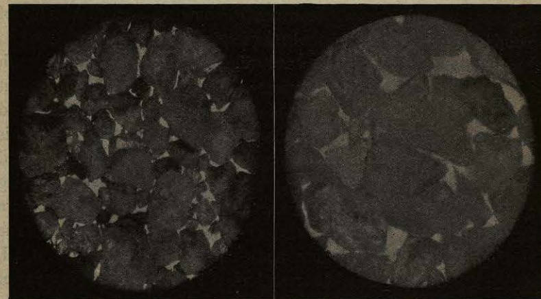
FIG. 64.—Natural Bank Sand.* No. 20 to No. 30 Sieves. (See p. 175)
