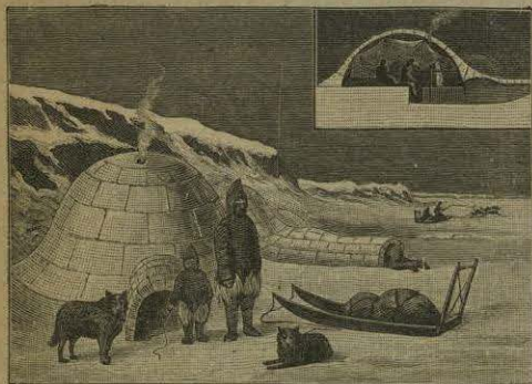
FIG. 525. — Eskimo winter home, or igloo. Entrance is by way of a small ice tunnel, through which wind does not easily enter.
