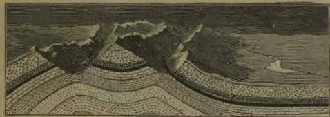
FIG. 191. — To illustrate how folding and denudation bring to light valuable mineral deposits. The black layer may represent a bed of coal. If the strata were horizontal, it might be deeply buried; but folding has raised it, and deep mountain valleys have exposed it to the air.
