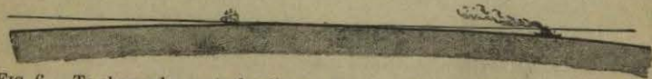
FIG. 6. — To show why part of a distant ship is hidden. The straight line is the line along which a man on the deck of the sailing vessel would look.
